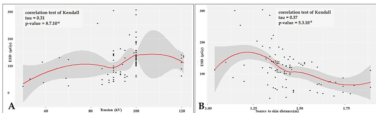
**Figure 3: Variation of the ESD according to the voltage (A) and the source to skin distance (B).**
